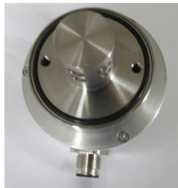
Figure 6: Mounting holes for sensor A19-S
