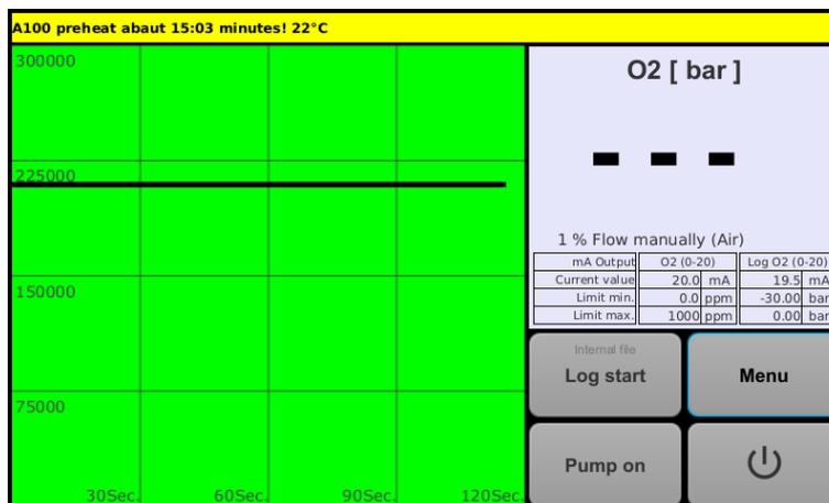
As long as the sensor temperature is below the target value, the measured value is shown as "- - -". The info line displays the current status of the heating process on a yellow background.
