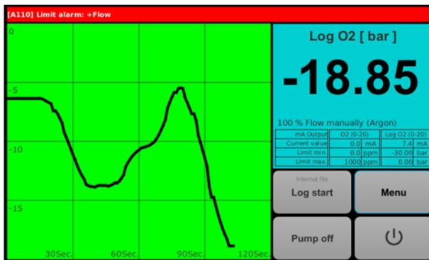
Measured value display and touchpad for selecting the measured value
