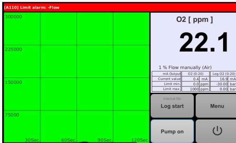
The start screen may display an alarm message in the info line on a red background. The alarm message can be removed by entering suitable alarm limits (see section "Alarms") and if the measured value lies within these limits.
