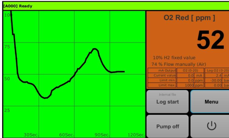
Example of the display showing a 0 - 1000 ppm range trend without band alarm
