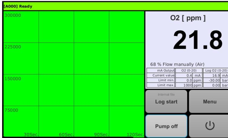
After the heating up phase, the measuring unit will display the measured oxygen value. In this case the info area shows: "Ready" while the background colour is green. A stable measured value is reached 15 minutes after the heating up process has been completed.
