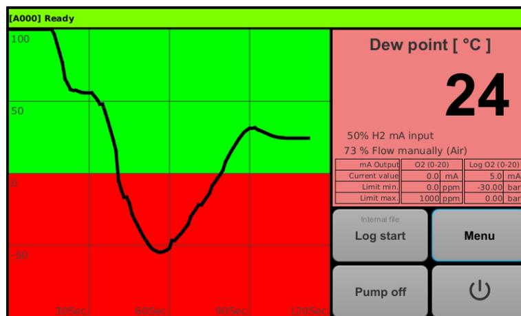
*Example of the display showing a -100 to +100 degree range trend with band alarm*
