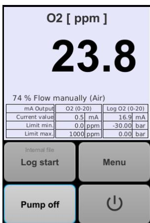
Touch pad for selecting measured values and measuring functions
