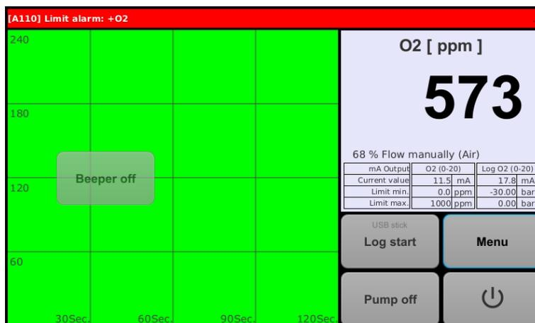
In case the beeper is activated and an alarm pending, the diagram area will display "Beeper Off"
