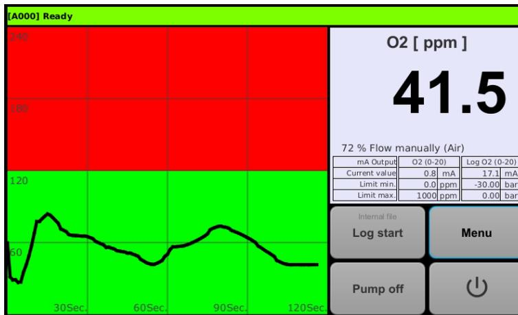
Example of the display showing a 0-240 ppm O<sub>2</sub> trend with band alarm
